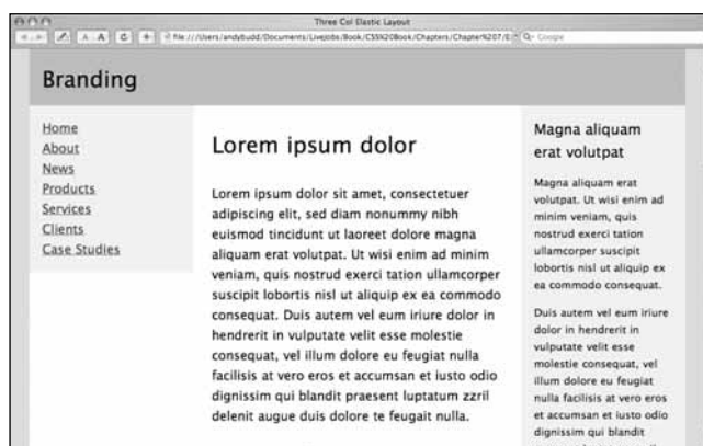
Figure 7-8. Elastic layout after the text size has been increased a few times
